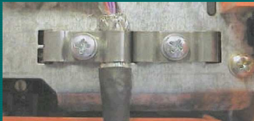
Connect the shield to the electronics shield clamp of the inverter 在变换器的电路板上用线卡连接
