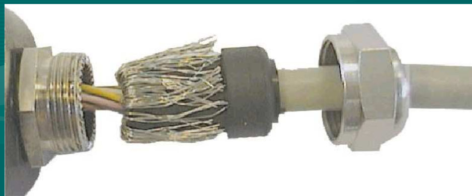
Connect the shield to the PG fitting of the encoder 编码器用屏蔽的PG接口连接
